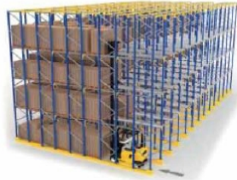
驶入式/通廊式货架系统 Drive-in / drive through racking
